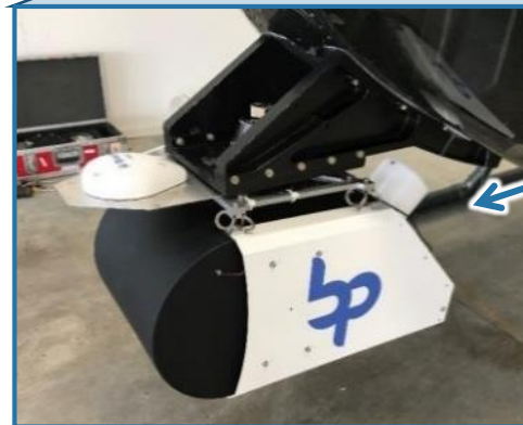
Integrated 3D Lidar and Gas Sensor
